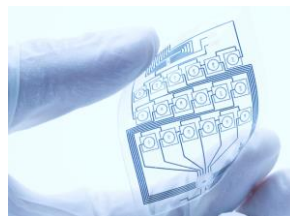
Figure 1 : Application of Conductive Ink on the Flexible Substrate
